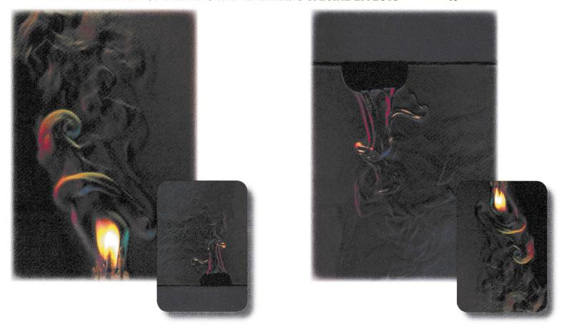
These two Schlieren photos, one of a candle flame, and one of an ice cube melting in water, show a remarkable similarity in the beautiful energy patterns that occur when hot and cold temperatures intermingle, regardless of the context. Rotating both photos 180 degrees and looking at them next to their opposites, shows us just how uncannily similar these patterns really are. We will find these patterns everywhere the various elements react to the cosmic forces at work in the world as we know it.
